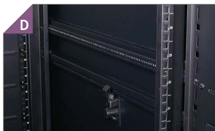
D Vertical rails of cabinets can be adjusted quarter-inch increments. Numbering system for U positions are provided for faster installation.
